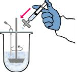
✓ Filter and collect remaining dissolution sample (about 1 mL) for analysis
