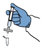
✓ Discard filter, re-attach syringe to cannula
